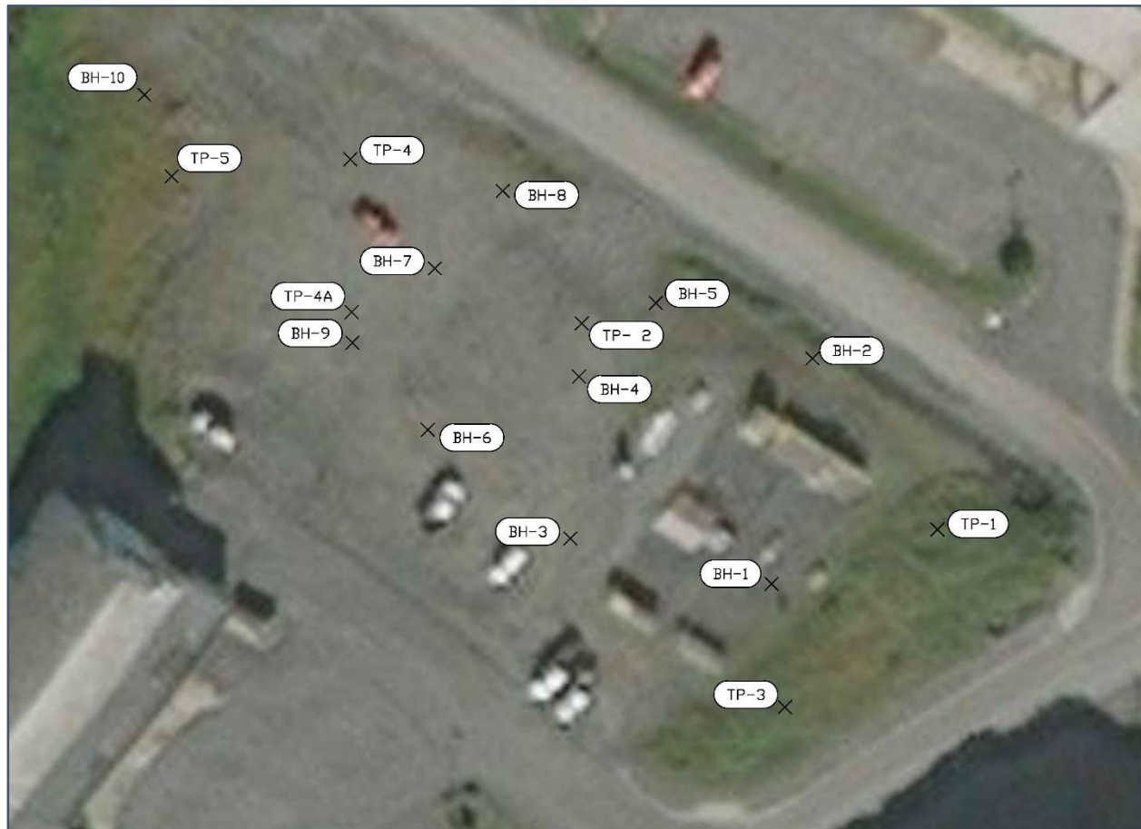
Figure 3-3-1. As-Built Borehole Locations
